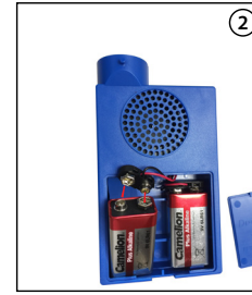
Ensure placement is matching battery (+ positive & - negative)
