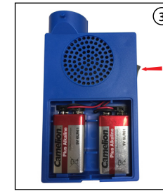
Insert securely into battery compartment & switch on to test power
